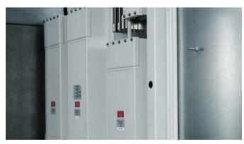
The high capacitances between the lines and ground require special protective measures. If there are no product-specific requirements, protection with a secondary ground wire (cross section min. 10 mm²) in accordance with EN 50178, is necessary. For this purpose, the filter case has connecting bolts at each end. Resistors are incorporated in the filter to discharge capacitors after shut-down.
