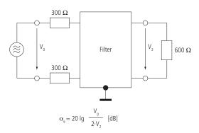
Symmetrical measurement circuit with  $Z_i = 600 \ \Omega$
