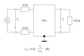
Symmetrical measurement circuit with  $\rm Z_{L}=100~\Omega$
